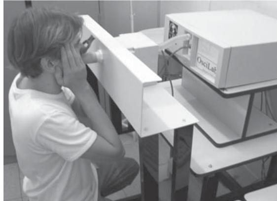
Figure 1 - Positioning of a volunteer during the test carried out through the use of the forced oscillation technique. Note the nasal clip and the use of the support to reduce the effect of the upper airways
