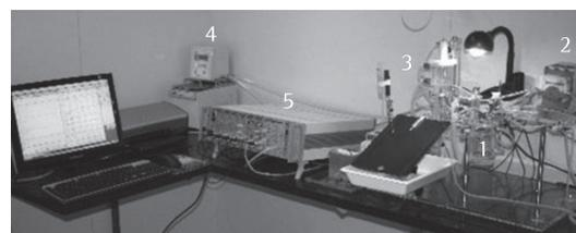
**Figure 1** - IL-2 Isolated Perfused Rat or Guinea Pig Lung System. 1) negative pressure chamber; 2) connected perfusion roller pump; 3) blood reservoir and membrane deoxygenator; 4) water heater in which water circulates around the entire perfusion system to maintain temperature; and 5) data acquisition module for acquiring data on hemodynamics, respiratory mechanics, and blood gas analysis (pH, PaO<sub>2</sub>), with transducers and a volume ventilator coupled to a personal computer.
