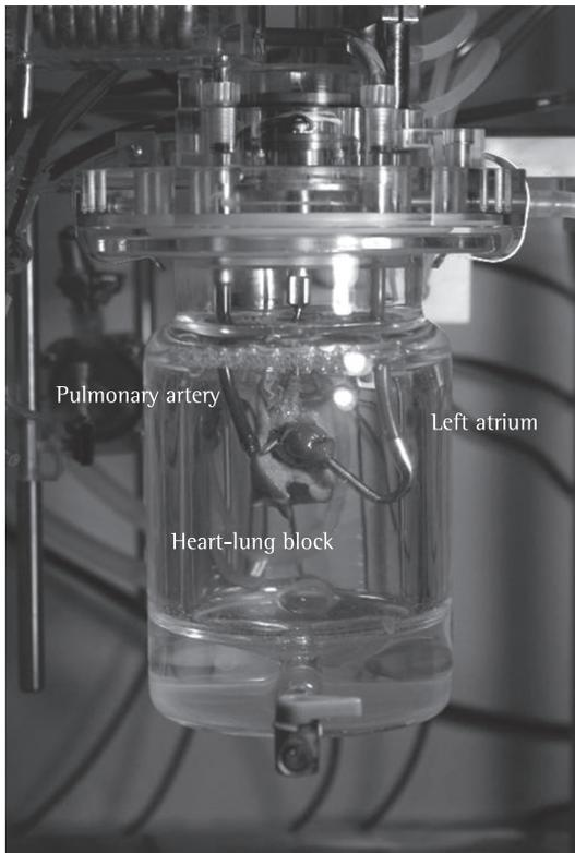
**Figure 2** - Negative pressure chamber containing the heart-lung block. The heart-lung block is placed within the negative pressure chamber and connected to the ventilation outlet, being perfused through the pulmonary arterial cannula and drained through the left atrial cannula.
